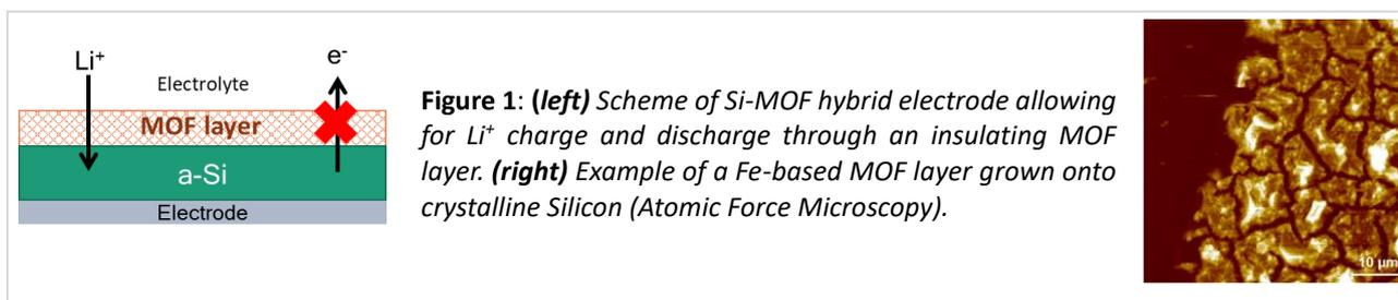
**Figure 1:** (left) Scheme of Si-MOF hybrid electrode allowing for  $\text{Li}^+$  charge and discharge through an insulating MOF layer. (right) Example of a Fe-based MOF layer grown onto crystalline Silicon (Atomic Force Microscopy).
